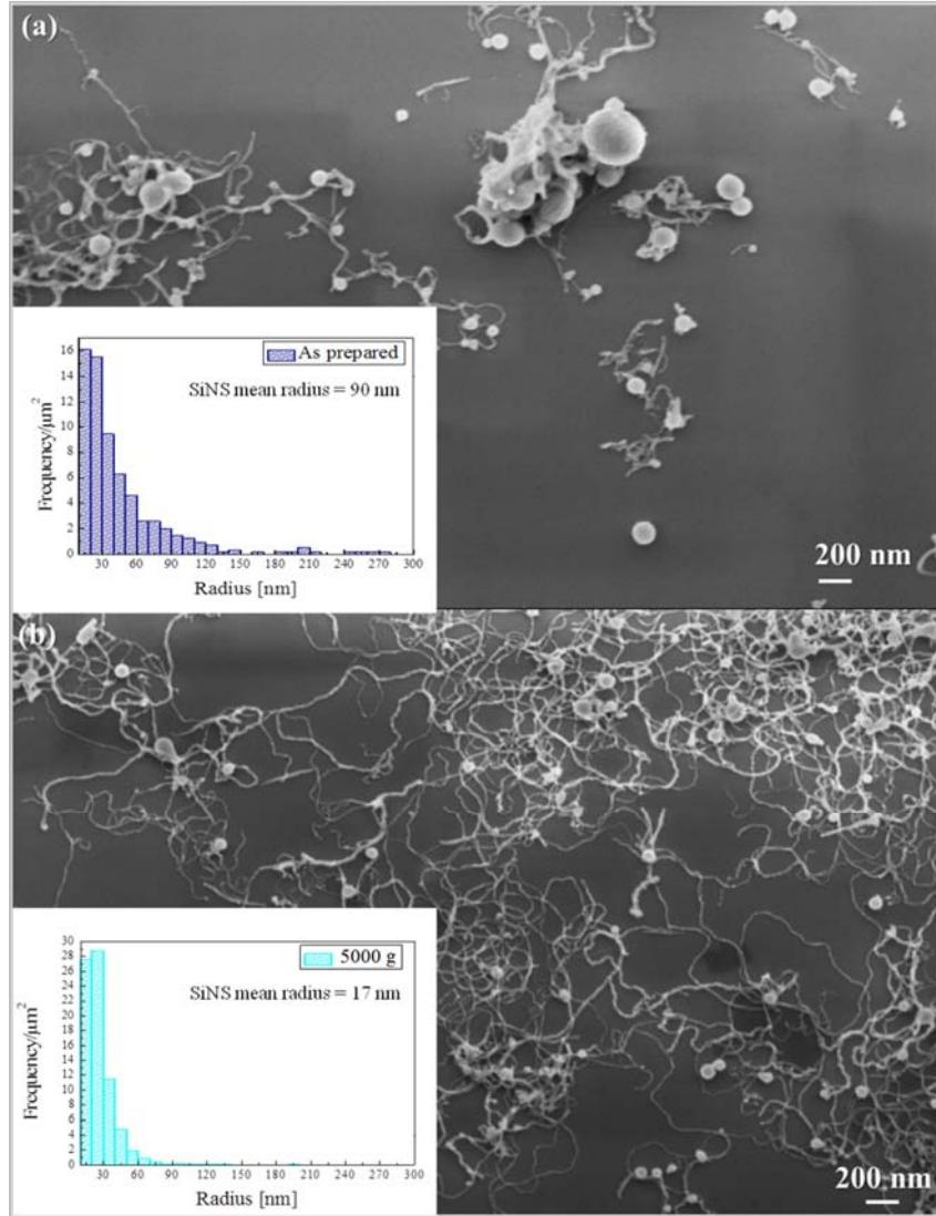
**Figure 5.3.** Typical SEM image depicting (a) the as-collected sample and (b) the sample centrifuged at 5.000 g. In the inset, the corresponding Si spheres size distributions are also shown.
