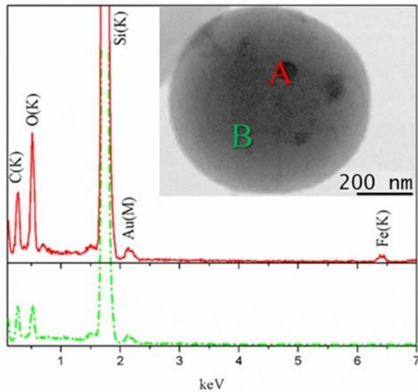
**Figure 4.14.** STEM-EDX spectra acquired in correspondence of a dark spot on the surface of the SiNS (point A in the STEM image) and above a no-contrast region, like the point B. The STEM-EDX spectrum acquired at the point A shows that although iron is present, no NW growth was induced.
