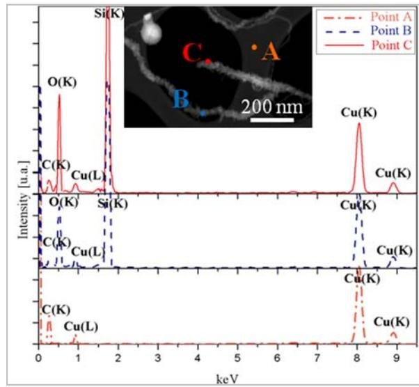
**Figure 4.7.** Typical STEM-EDX spectra relative to the 95% of the ICP-SiNWs. The spectra were acquired on the carbon lacey TEM grid (A, orange color), along the SiNWs (B, blue color), on the top of the SiNWs (C, red color), as shown in the corresponding HAADF-STEM image.
