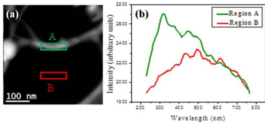
**Figure 3.9.** (a) Dark field TEM image of a single ICP-SiNWs, from which (b) optical emission has been detected via CL spectroscopy.
