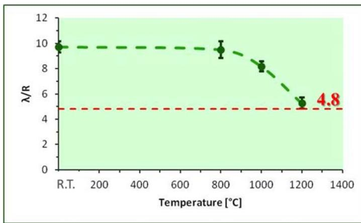
**Figure 6.6.** Graph showing the trend of the ratio  $\lambda/R$  in samples annealed at different temperatures; at 1200°C, the value of  $\lambda/R$  is in agreement with the theoretical value of 4.8, represented by the red line.
