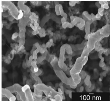
**Figure 2.10.** Typical Scanning Electron Microscopy (SEM) image of SiNWs synthesized via CVD [Hofmann03].
