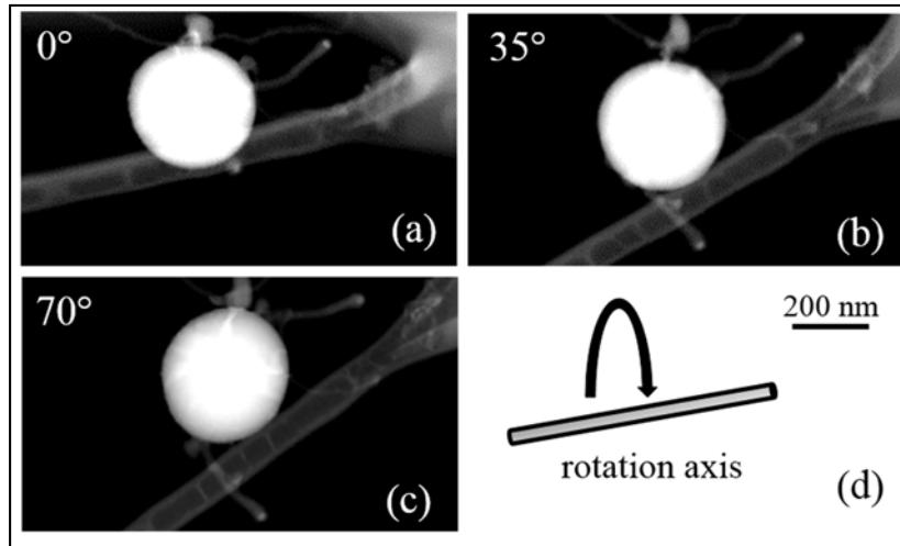
**Figure 4.12.** HAADF-STEM micrographs of a SiNS with two connected SNWs, acquired at (a) 0°, (b) 35° and (c) 70° of sample rotation along the rotation axis shown in (d).
