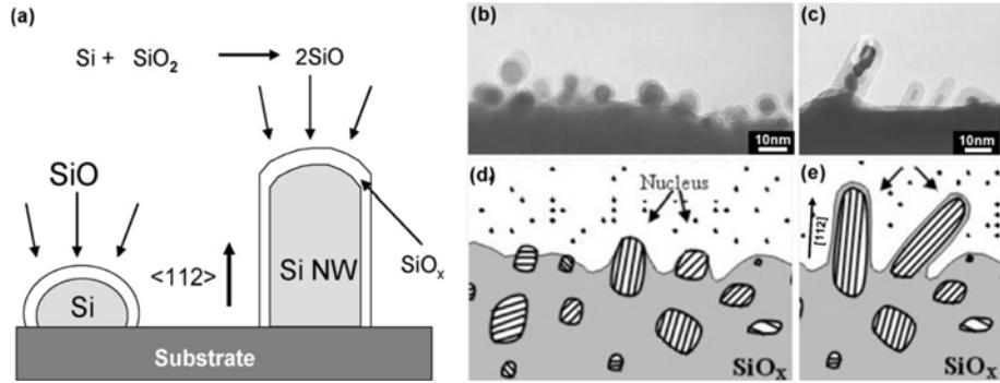
**Figure 2.8.** (a) Sketch of the OAG mechanism. (b) TEM image of Si nanoparticles precipitate from the decomposition of SiO matrix. (c) The nanoparticles in a preferred orientation grow fast and form nanowires. (d, e) OAG model for the nucleation and early stages of the growth of SiNWs [Lee00].
