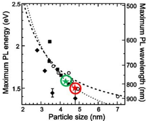
**Figure 4.18.** Theoretically predicted correlation between the size and the PL energy in SiNCs [Ledoux00], whilst the green and red stars correspond to the experimental value obtained for SiNCs having mean diameter  $\sim 3.2$  nm and  $3.8$  nm, respectively.
