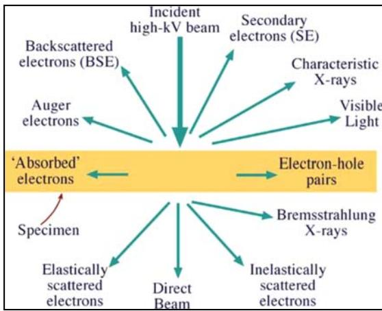
**Figure 3.4.** Signals generated by the electron-matter interaction [Williams09].
