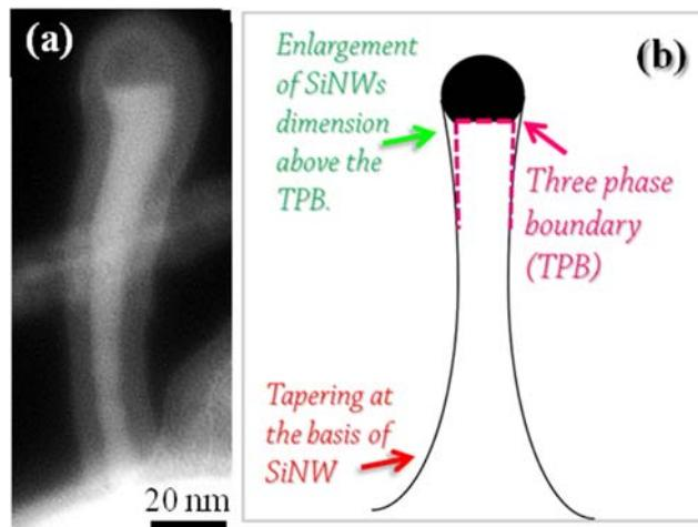
**Figure 4.15.** (a) Typical EFTEM image of an ICP-SiNW grown via VLS mechanism, which presents an enlargement of the diameter at the top, in correspondence of the Fe catalyst-NW interface; (b) sketch of a SiNW where the effect of the tapering and of the surface diffusion above the catalyst particle are evident.
