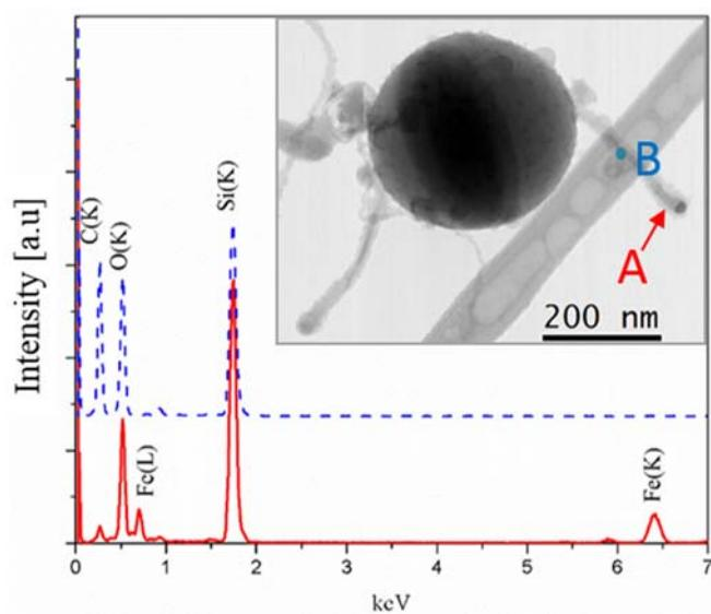
**Figure 4.10.** Typical STEM-EDX spectra exhibited by ~5% ICP-SiNWs, as the one displayed in the BF TEM image in the inset. The (A) and (B) locations are also shown.
