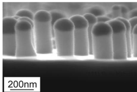
Figure 2.11. Typical SEM image of MBE-grown SiNWs [Schubert04].
