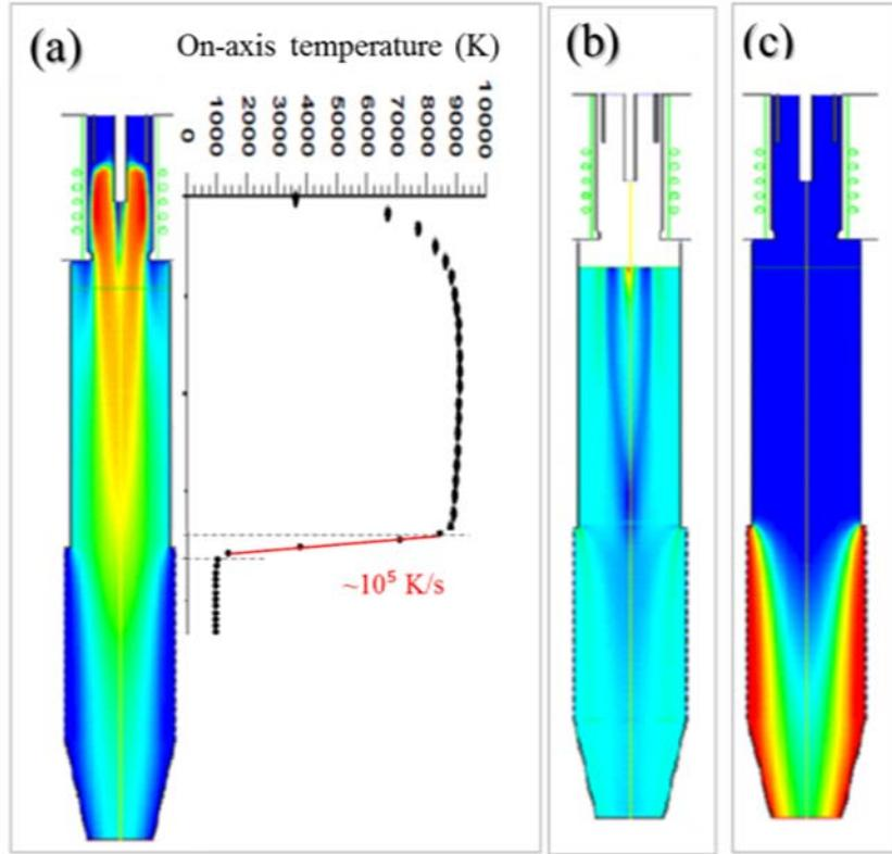
**Figure 3.2.** Numerical modeling regarding (a) the temperature distribution inside the plasma chamber, (b) the rate of temperature variation and (c) the distribution of the gaseous cold front having a quenching action [Guo10]. Temperature field (Red=10.000 K and Blue=350 K).
