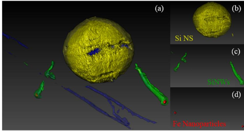
**Figure 4.13.** Volume reconstruction of the system formed of a SiNS and two SiNWs. The different areas of interest, namely the (b) SiNS, (c) the SiNWs and (d) and the Fe particles have been reconstructed separately and then combined in (a).
