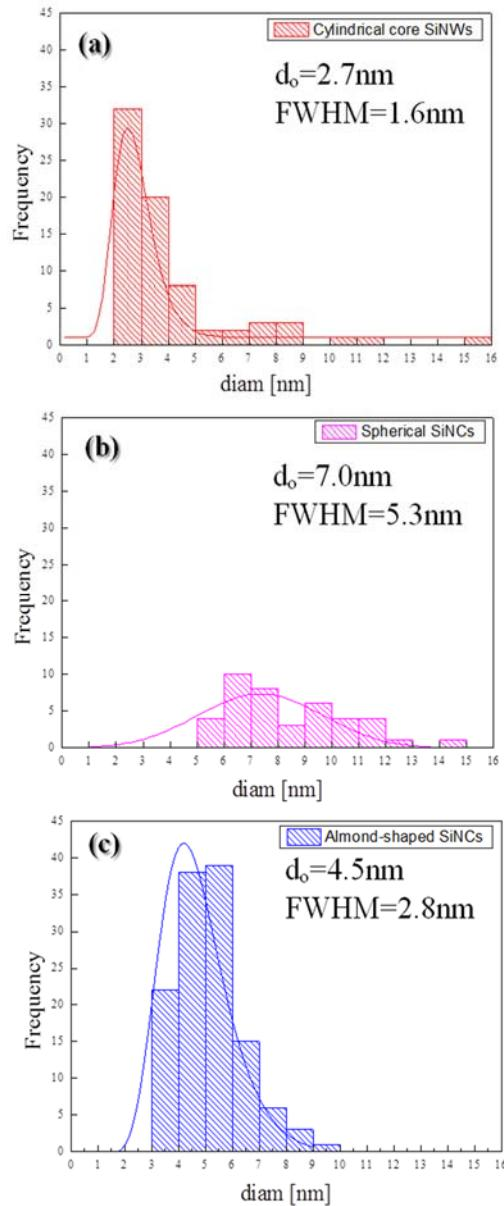
**Figure 4.5.** Diameter distributions relative to: (a) the cylindrical SiNWs, (b) almond-shaped SiNCs and (c) spherical SiNCs.
