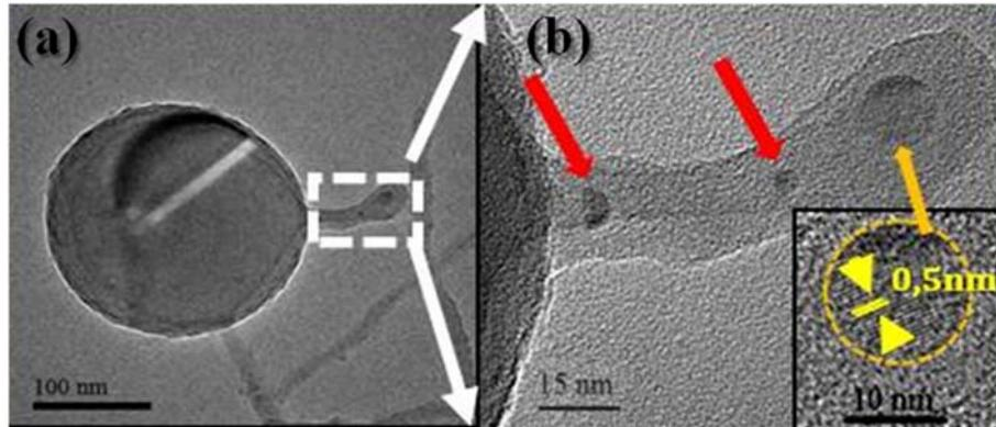
**Figure 4.9.** (a) Bright Field TEM image showing a SiNS, whose core generates three perpendicular NWs. (b) Enlarged image on the NWs. The arrows indicate three small nanoparticles at the end of each wire; in particular the top particle, enlarged in the inset, presents interference fringes corresponding to 0.5 nm interplanar distance.
