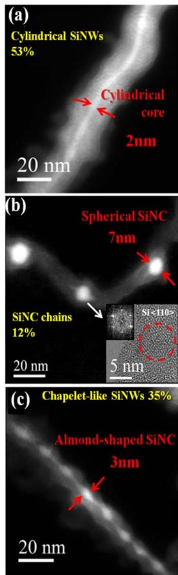
**Figure. 4.4.** Energy Filtered TEM acquired at 17 eV, showing the three internal configurations of ICP-SiNWs: (a) a cylindrical Si nanocore, (b) a chain composed of spherical SiNCs whose crystalline nature is clarified by the HRTEM in the inset and (c) chapelet-like wire composed by almond-shaped SiNCs connected by a very thin SiNW. Cylindrical SiNWs represent ~53% of the whole population, while the SiNC chains constitute ~12% and the "chapelet-like" are ~35%.
