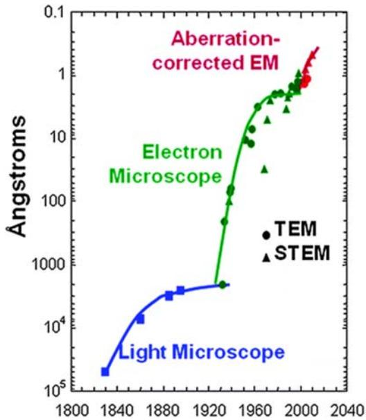
**Figure 3.3.** Trend of spatial resolution achieved in the last two centuries; thanks to the aberration-corrected TEM the sub-Å resolution is nowadays reachable. The resolution obtained via optical microscopy is also displayed for comparison [Pennycook14].
