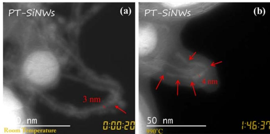
**Figure 6.1.** EFTEM images of (a) a cylindrical SiNW at  $t \sim 0$  and (b) the same SiNW after ~1 hour and 45 min: it can be seen that the SiNW broke up into Si crystalline fragments.
