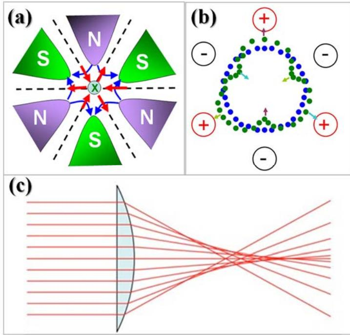
**Figure 3.5.** (a) Sketch of a hexapole magnetic lens; (b) deformation of the electron beam under the action of a hexapole; [Liao07] (c) Effect of the spherical aberration [Houdellier14].
