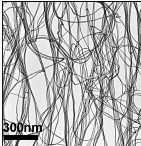
**Figure 2.13.** Typical SEM image of SiNWs grown via thermal evaporation [Zhang03].
