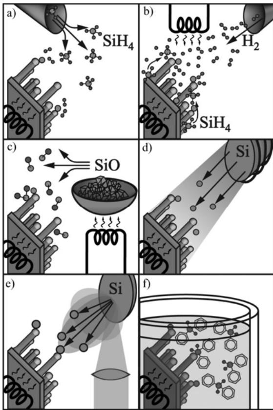
**Figure 2.9.** Schematic of the bottom-up techniques used for the synthesis of SiNWs: (a) Chemical Vapor Deposition, (b) Annealing in reactive atmosphere, (c) Thermal Evaporation of  $\text{SiO}$ , (d) Molecular Beam Epitaxy, (e) Laser Ablation, (f) Synthesis in solution [Schmidt09].
