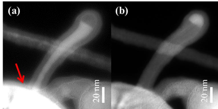
**Figure 4.11.** EFTEM images acquired at the plasmon energy loss of (a) Si, and (b) SiO<sub>2</sub>. The arrow indicates the structural connection between the Si core and the SiNS, as well as the continuity of the oxide shells of the SiNW and the SiNS.
