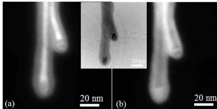
**Figure 7.2.** EFTEM images acquired at the plasmon energy losses of (a) Si and (b)  $\text{SiO}_2$  of two SiNWs having a dark particle at their tips, as shown in the inset.
