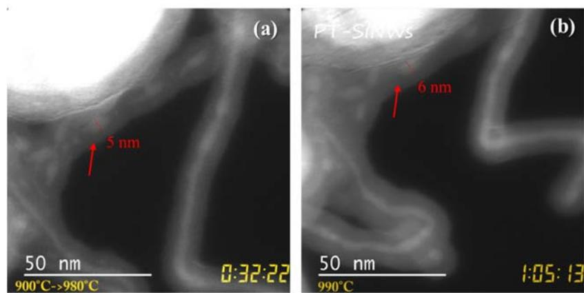
**Figure 6.210.** (a) EFTEM image of a chapelet-like SiNW subject to in-situ thermal annealing after ~30 minutes; (b) the same nanostructures after almost 1 hour show an evolution towards a SiNC chain morphologies.
