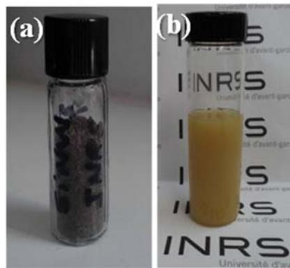
**Figure 4.1.** (a) Small amount of the “as-collected” Si powder found after the spheroidization process exploited in conventional ICP. (b) Solution prepared by dispersing the Si powder in isopropyl alcohol.
