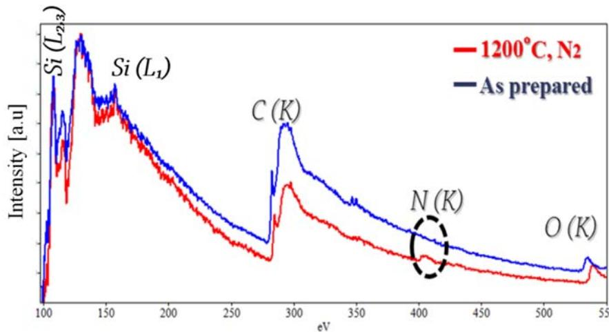
**Figure. 3.7.** High loss EELS spectra of ICP-SiNWs as-collected and annealed at 1200°C in N<sub>2</sub>, showing nitrogen incorporation the SiNWs after annealing.
