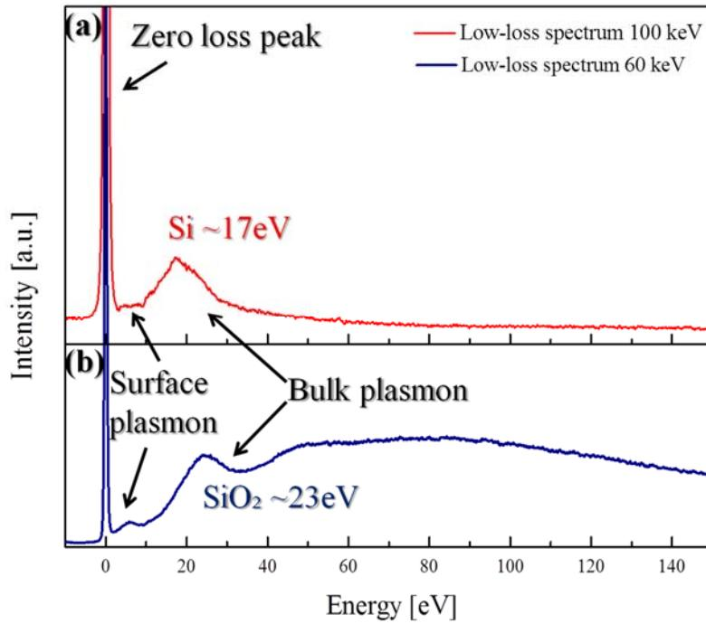
**Figure 3.6.** Low-loss EELS spectra of as collected ICP-SiNWs detected at 60 keV (blue line) and 100 keV (red line).
