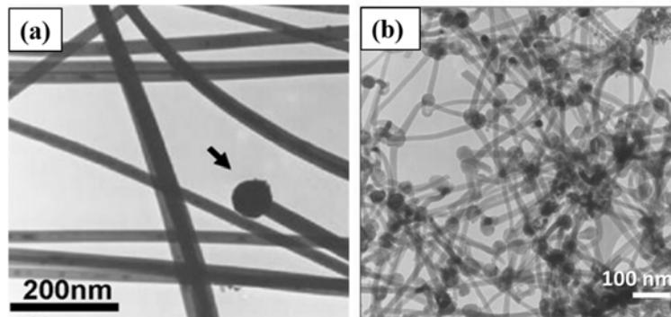
**Figure 2.12.** (a) SiNWs grown by means of laser ablation via the VLS mechanism, as indicated by the presence of particles at the top of the wires, as marked by the arrow [Wang08]. (b) SiNWs produced in bulk quantity via laser ablation technique [Morales98].
