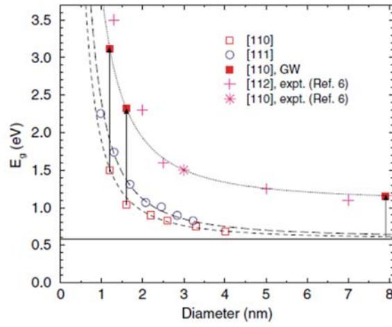
**Figure 1.9.** Local density approximation based calculations of the band gaps for [110] (empty squares) and [111] (empty circles) wires, and the GW-corrected gaps (filled squares) for the two thinnest [110] wires, compared with the measured gaps for [112] wires (+) and a [110] wire (\*). The dotted, dashed, and continuous lines are fitted to the data points [Zhao04].
