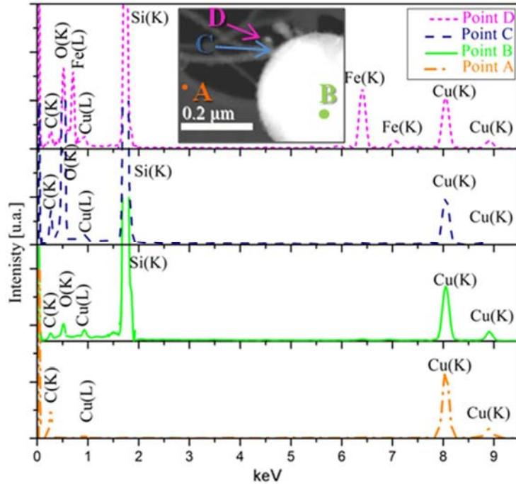
**Figure 3.8.** STEM-EDX spectra acquired at different points of ICP-SiNWs, as shown in the dark field image reported in the inset.
