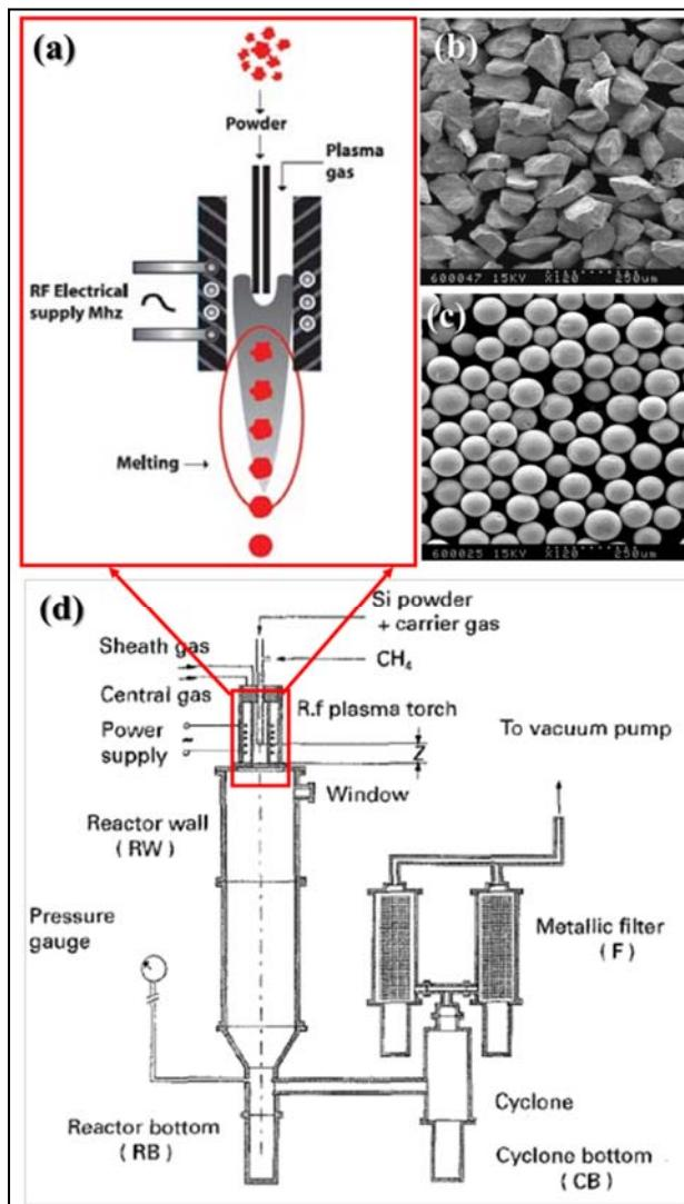
**Figure 3.1.** Illustration of the spheroidization system for spherical micropowder synthesis: a Si rough powder (a) is inserted in the plasma tube (c) as a feedstock for the production of high-quality spherical micropowders (b). The reactor for micropowder synthesis is sketched in (d). [www.tekna.com]
