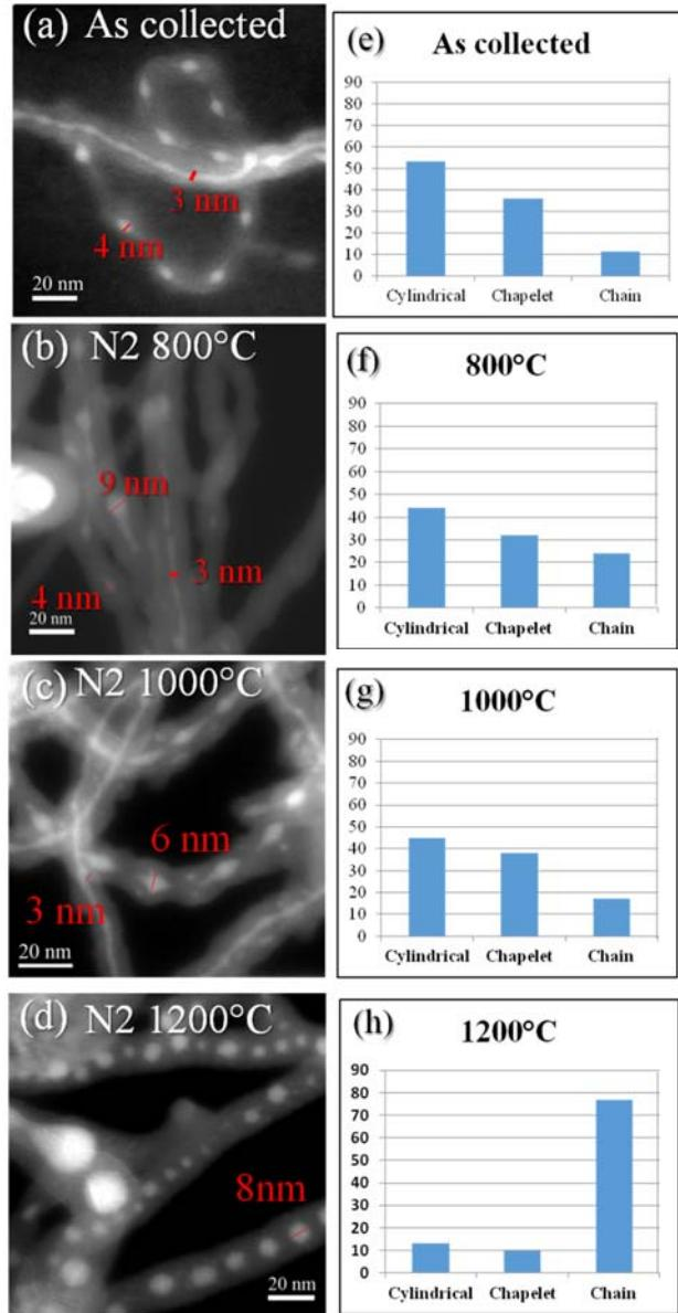
**Figure 6.3.** EFTEM images of (a) the as-collected sample and the samples annealed at (b) 800°C, (c) 1000°C and (d) 1200°C in N<sub>2</sub> for 1 hour. (e-h) Corresponding statistical distribution of the occurrence of the three different SiNW morphologies.
