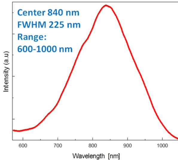
**Figure 3.12.** The typical PL spectrum acquired from the as collected SiNWs is centered in the visible-near IR range.
