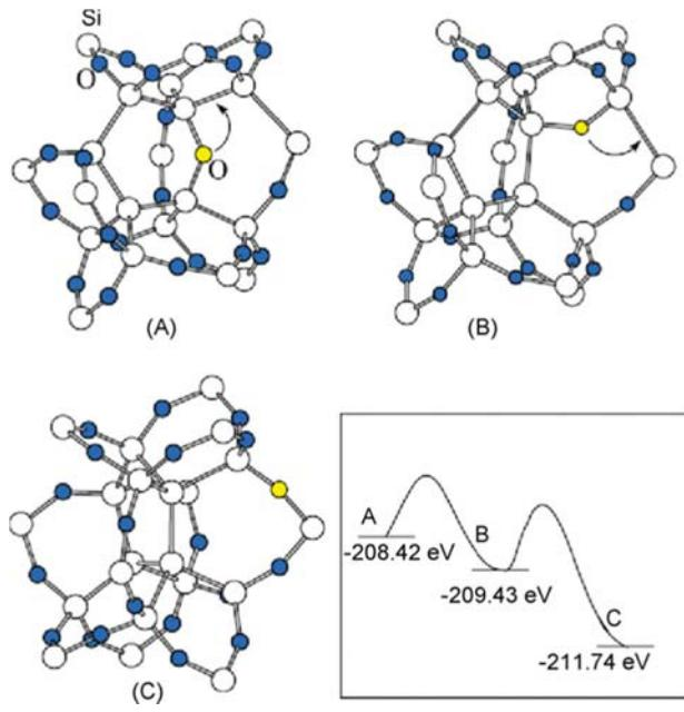
**Figure 2.7.** Isomers of the SiO clusters with the O atom (in yellow) in different locations: (a) at the center of the cluster, (b) at intermediate position, (c) at the cluster surface. The associated binding energies for each configuration is also displayed [Wang08].
