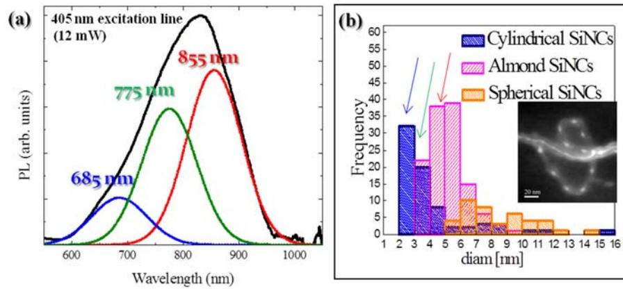
**Figure 4.16.** (a) Representative PL spectrum of the as-collected SiNWs as long as its deconvolution into three main components; (b) illustration of the diameter distributions related to the three different morphologies in the as-collected powder.
