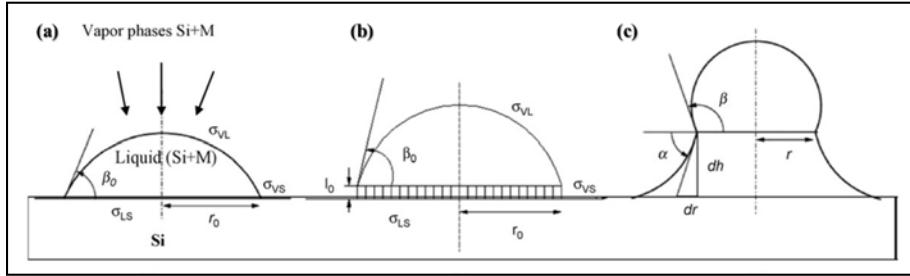
**Figure 2.3.** (a) Condition at  $t=0$ ; (b) early stage of SiNW growth, where the first Si crystalline monolayer is formed; (c) equilibrium condition for SiNW growth [Wang08].
