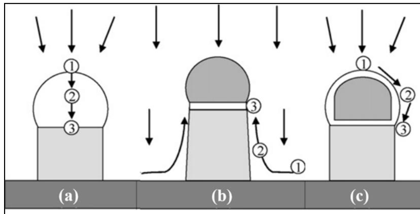
**Figure 2.4.** (a) Adsorption of Si atoms in the droplet; (b) diffusion of Si atoms on the metallic particle and incorporation of Si at the liquid-solid interface; (c) diffusion of the Si atoms on the substrate and incorporation at the SiNW flanks [Wang08].
