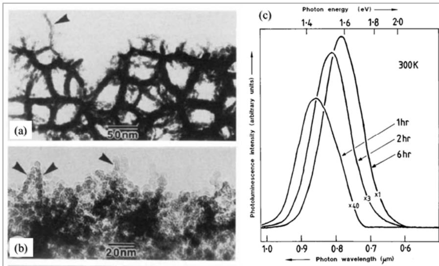
**Figure 1.4.** (a and b) Bright field TEM images of porous Si with decreasing porosity: (a) non-luminescent sample and (b) luminescent sample. (c) PL emission of porous Si synthesized by increasing the anodization time and, thus, the porosity [Cullis97].
