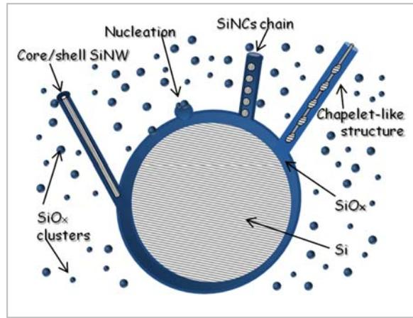
**Figure 4.8.** Sketch of SiNW formation via the OAG mechanism, illustrating the nucleation operated by a Si suboxide cluster on the silica shell of the SiNS, which represents the substrate for SiNW growth. According to this model, the formation of SiNC chains or chapelet-like nanostructures is also possible [Zhang03].
