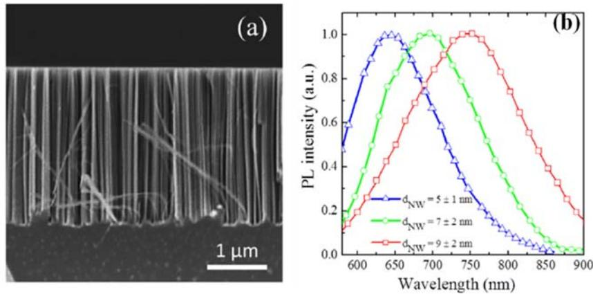
**Figure 1.7.** (a) SEM image of SiNWs synthesized via metal assisted chemical etching; (b) PL emission of SiNWs with different size [Irrera12].
