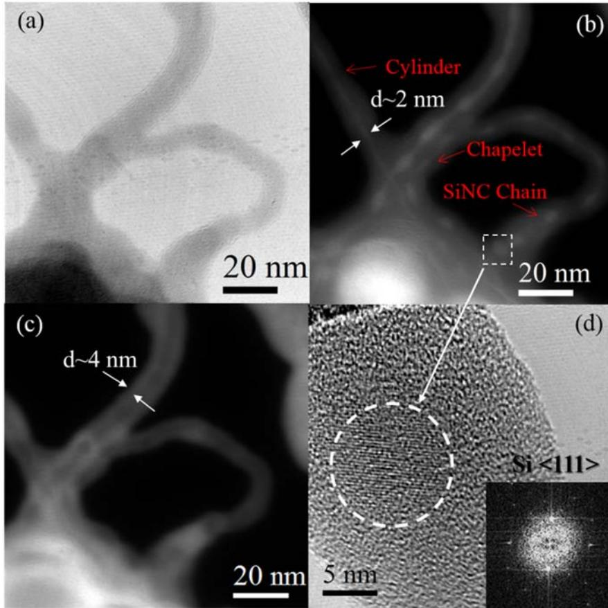
**Figure 7.1.** TEM images of SiNWs reproduced via intentional ICP synthesis: (a) BF TEM; (b) EFTEM image acquired at the Si plasmon energy loss; (c) EFTEM image acquired at the  $\text{SiO}_2$  plasmon energy loss; (d) HRTEM depicting a spherical SiNC with the corresponding Fast Fourier Transform.
