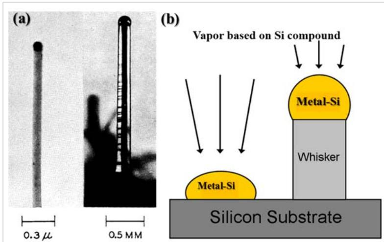
**Figure 2.1.** (a) Si whiskers synthesized via VLS mechanisms, firstly reported by Wagner and Ellis. [Wagner64]. It can be noted that the lateral dimensions were quite big, up to 0.2 mm. (b) Schematic of the 1D Si nanostructures growth via VLS.
