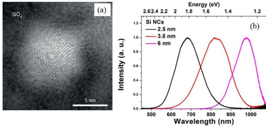
**Figure 1.5.** (a) Energy Filtered TEM image of a  $\sim 9$  nm wide SiNC embedded into a  $\text{SiO}_x$  matrix [Iacona04]. (b) Normalized PL intensity of SiNCs with different size. The wavelength shifts towards the blue while decreasing the SiNC diameter [Wen15].
