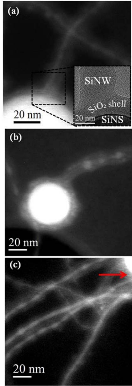
**Figure. 4.6.** EFTEM images acquired at 17 eV showing that (a) cylindrical SiNWs, as well as (b) SiNC chains and (c) chapelet-like SiNWs originate from the silica shell covering the SiNSs, as indicated by the arrow in (c) and better detailed in the inset of (a).
