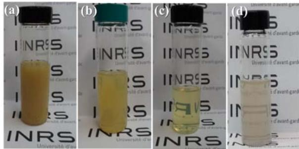
**Figure 5.1.** Comparison of solutions (a) before centrifugation and after centrifugation at (b) 1.000 g, (c) 5.000 g and (d) 15.000 g.
