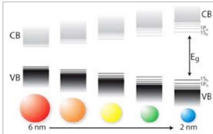
**Figure 1.6.** Illustration of bandgap enlargement and discretization of the energy levels induced by the decreasing of the size.
