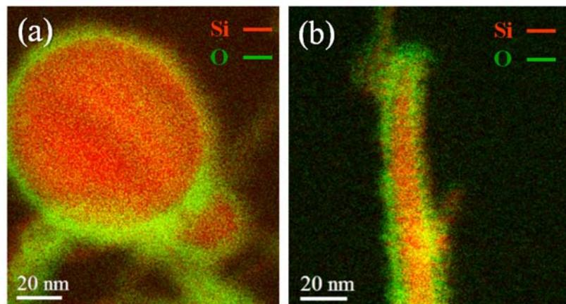
**Figure 4.3.** Energy Filtered TEM of (a) a SiNS and (b) a SiNW, demonstrating a structure of ICP-Si nanostructures made up of a Si core (in red) and a SiO<sub>2</sub> shell (in green).
