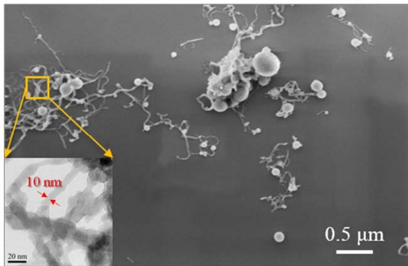
**Figure. 4.2.** Typical SEM image of the ICP-Si nanopowder based sample, showing an array of nanowires and nanospheres. A typical bright field TEM of the nanowires is depicted in the inset.
