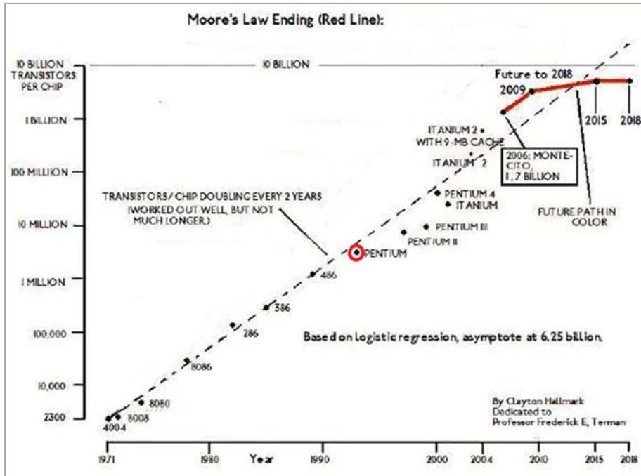
**Figure 1.2.** Illustration of Moore's law: the dashed line shows the doubling of transistors in a chip every two years. We can see that between 1990 and 2000 Moore's law had an inflection point. In general, Moore's trend is forecasted to slow down in the next years [webinfo].
