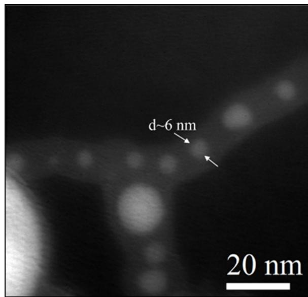
**Figure 7.3.** Representative EFTEM image of the sample annealed at 1200°C in N<sub>2</sub> acquired at the Si plasmon energy loss, showing the SiNC chain configuration.
