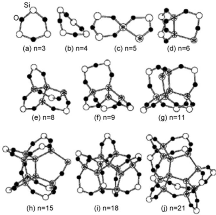
**Figure 2.5.** Early stages of SiO-like clusters aggregation, which evolves from the buckled-ring configuration (a and b) to the formation of a Si core surrounded by a silicon oxide shell (c-j). The open circles containing stars in (c) represent the Si core surrounded by a silicon oxide shell. The crystalline arrangement is most favored after  $n=18$  (i) [Wang08].
