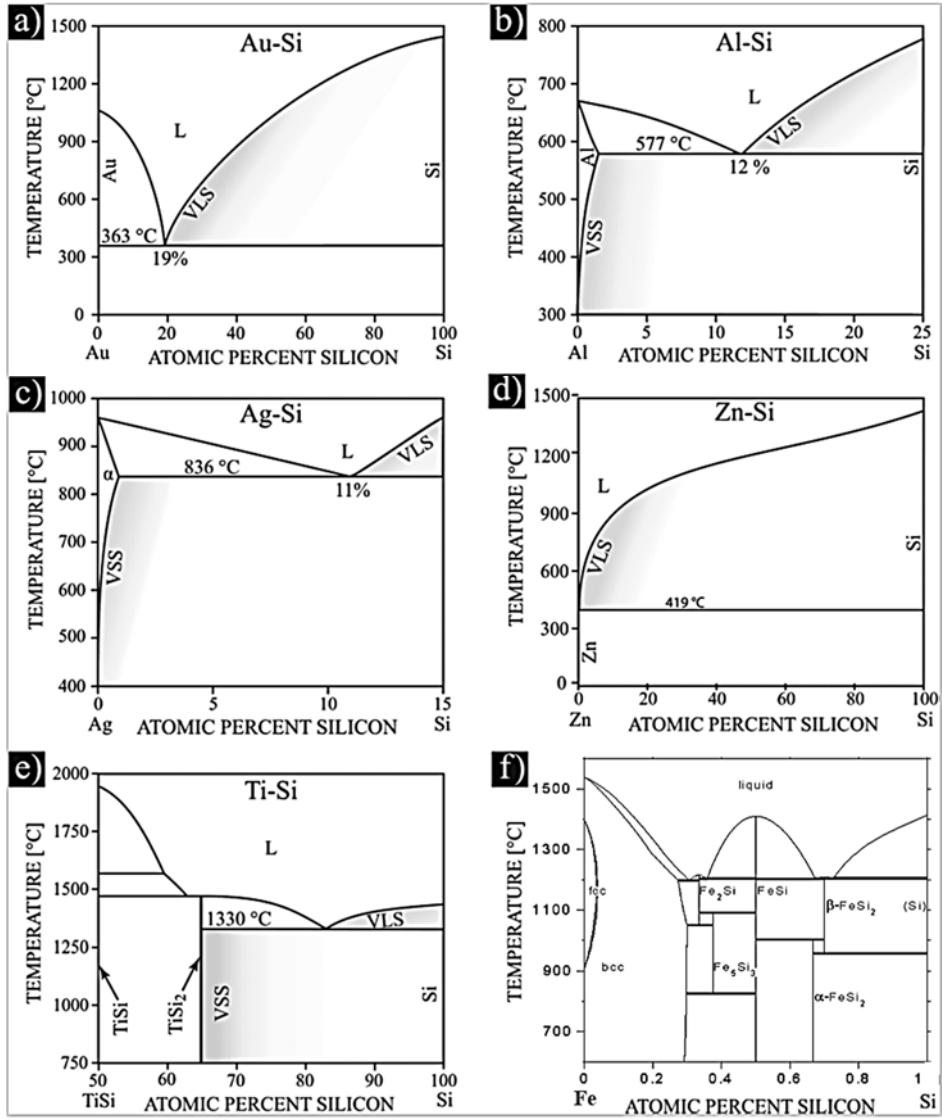
**Figure 2.2.** Phase-diagrams of some metal-Si alloys exploited for the synthesis of SiNWs: (a) Au, (b) Al, (c) Ag, (d) Zn, (e) Ti [Schmidt10] and (f) Fe [PDDatabase].
