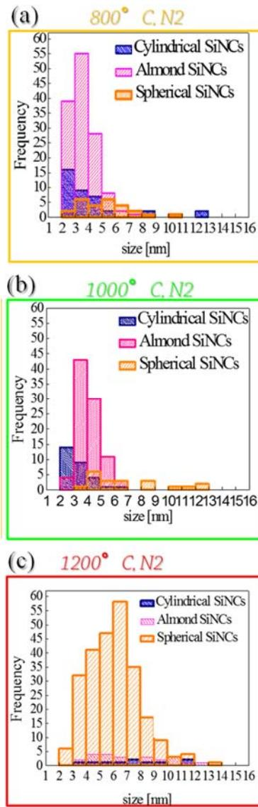
**Figure 6.4.** Size distributions of the diameters of Si cylinders (blue color), almond-shaped SiNCs (magenta color) and spherical SiNCs (orange color) in the samples annealed at: (a) 800°C, (b) 1000°C, (c) 1200°C.
