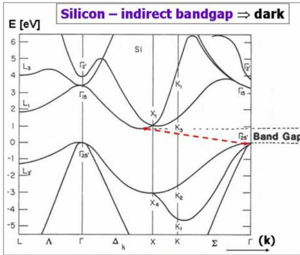
**Figure 1.3.** Energy band diagram of Si.
