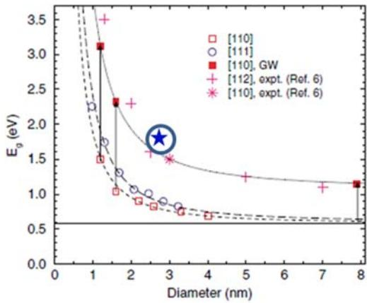
**Figure 4.17.** Theoretically predicted correlation between the size and the PL energy in SiNWs [Zhao04], whilst the blue star corresponds to the bandgap expected cylindrical ICP-SiNWs having mean diameter ~ 2.7 nm.
