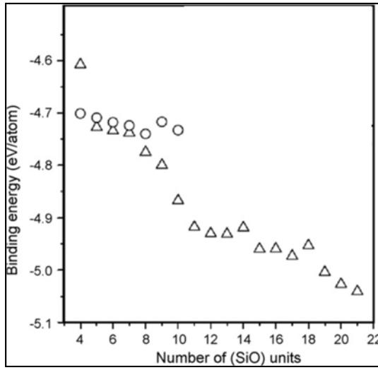
**Figure 2.6.** Binding energy (eV/atom) of  $(\text{SiO})_n$  clusters vs. the number  $n$  of SiO units. The triangles are  $(\text{SiO})_n$  with the Si-core structure surrounded by a silicon oxide sheath and open circles are those with buckled-ring structure [Wang08].
