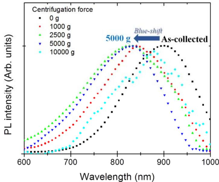
**Figure 5.2.** Normalized PL spectra of the as-collected sample and of samples centrifuged at different accelerations: 1'000 g, 2'500 g, 5'000 g and 10'000 g.
