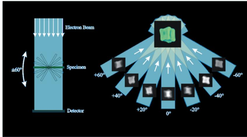
**Figure 3.11.** Sketch of the working principle of the electron tomography sample holder.
