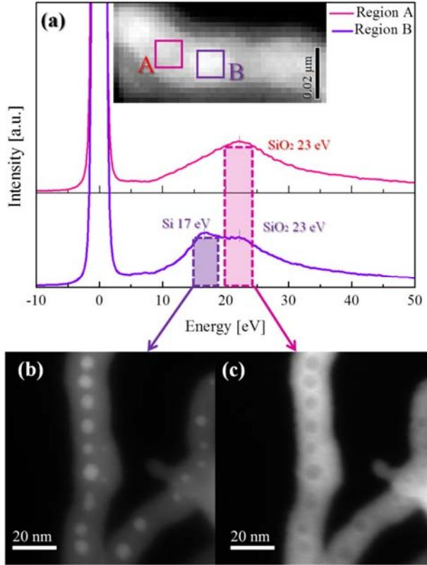
**Figure 3.8.** (a) Low-loss EELS spectra acquired in SI mode, corresponding to two different region of the nanostructure depicted in the HAADF image of the inset. (b) and (c) EFTEM images at the energy plasmon loss of Si and SiO<sub>2</sub>.
