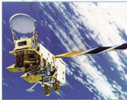
**Figure 1-3**      **Advanced Microwave Scanning Radiometer (AMSR), (Ulaby et al., 2014)**
