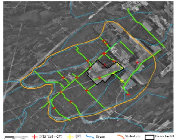
Figure 2 General context of the study area. Green lines represent the GPR surveys, red crosses represent the wells and the black lines represent the landfill.
