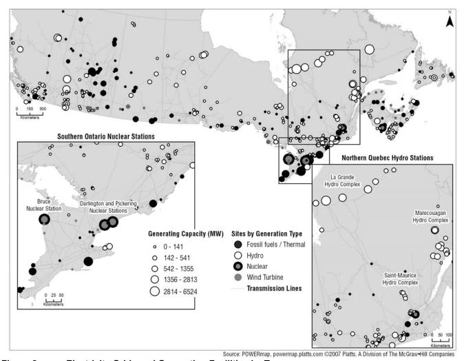
Figure 2 Electricity Grids and Generation Facilities by Type
