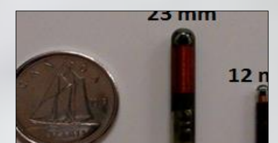
Figure 4 HDX Passive Integrated Transponder used to mark the fish
