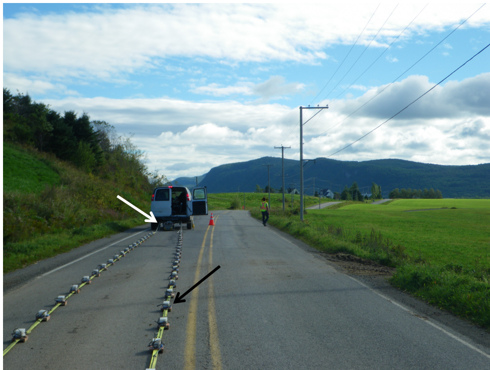
Figure 2.1 Landstreamer with three components geophones (black arrow) and small vibrating source (white arrow) towed by a vehicle during seismic data acquisition.
