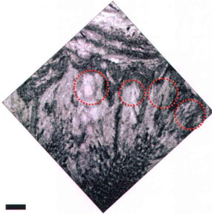
Figure 24. Post mortem image of Zone II. Red circles outline some of the dendrites with tips with radii from left to right  $\sim 1.8 \mu\text{m}$ ,  $\sim 1.3 \mu\text{m}$ , and  $\sim 1.6 \mu\text{m}$ . The scale bar is  $2 \mu\text{m}$ .
