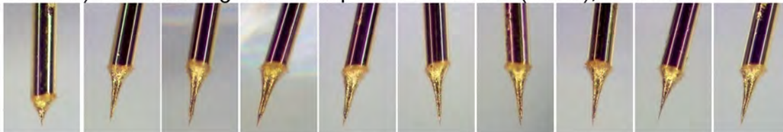
Figure 3.2.9: Optical images of the etched tips from series 1 to 5. The gold wire has a diameter of 100 \mu\text{m} and can be used as scale bar.
