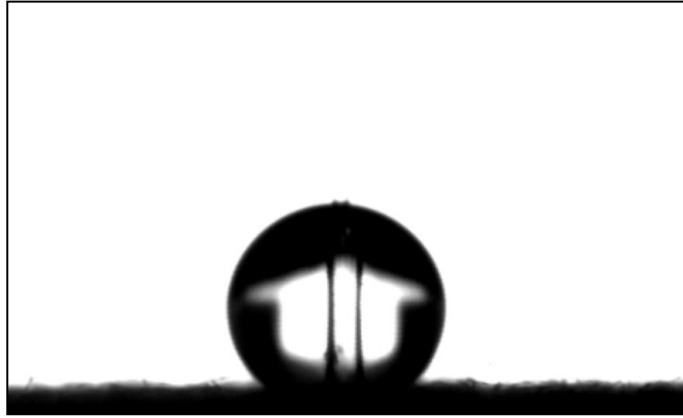
Figure 2.8 : Water drop on the surface of N 15 / T 00 cathode.
