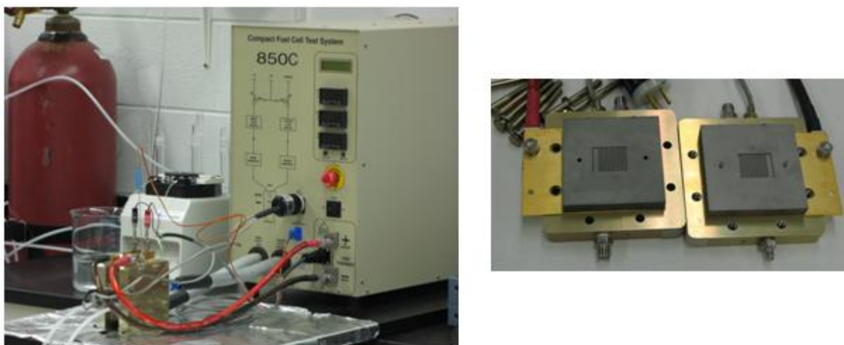
Figure 2.13: Fuel cell station and fuel cell test fixture.
