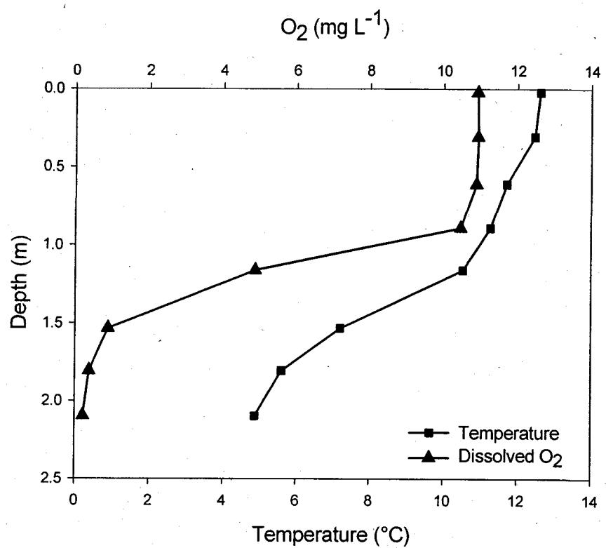
**Figure 9** Vertical profile temperature and oxygen concentration in the subarctic pond KWK1 performed at time of the day on June 28, 2007.
