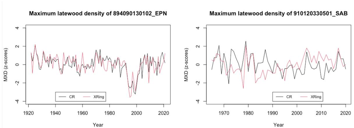
**Figure 7.** Comparison of maximum latewood density measured using CooRecorder (CR) and XRing for two selected coniferous species. Note: time series are z-scored due to the unknown value conversion in CR.
