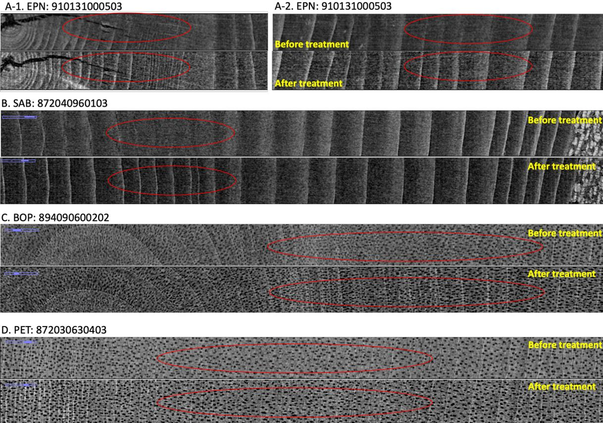
**Figure 8.** Effect of resin extraction (90% ethanol treatment) on the clearness of tree-ring boundaries.
