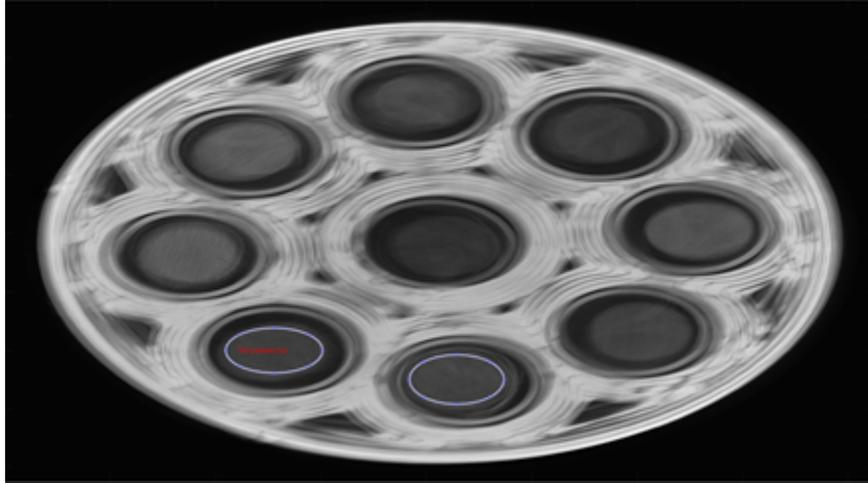
**Figure 4.** Extraction of wood cores from a 3D scan of 9 wood cores. Note blurry view is normal because the DensitometryToolbox displays a stacked average across the height. The blue circles indicate cores to be extracted. One needs to specify sample IDs orderly in the Excel sheet provided along with the DensitometryToolbox.
