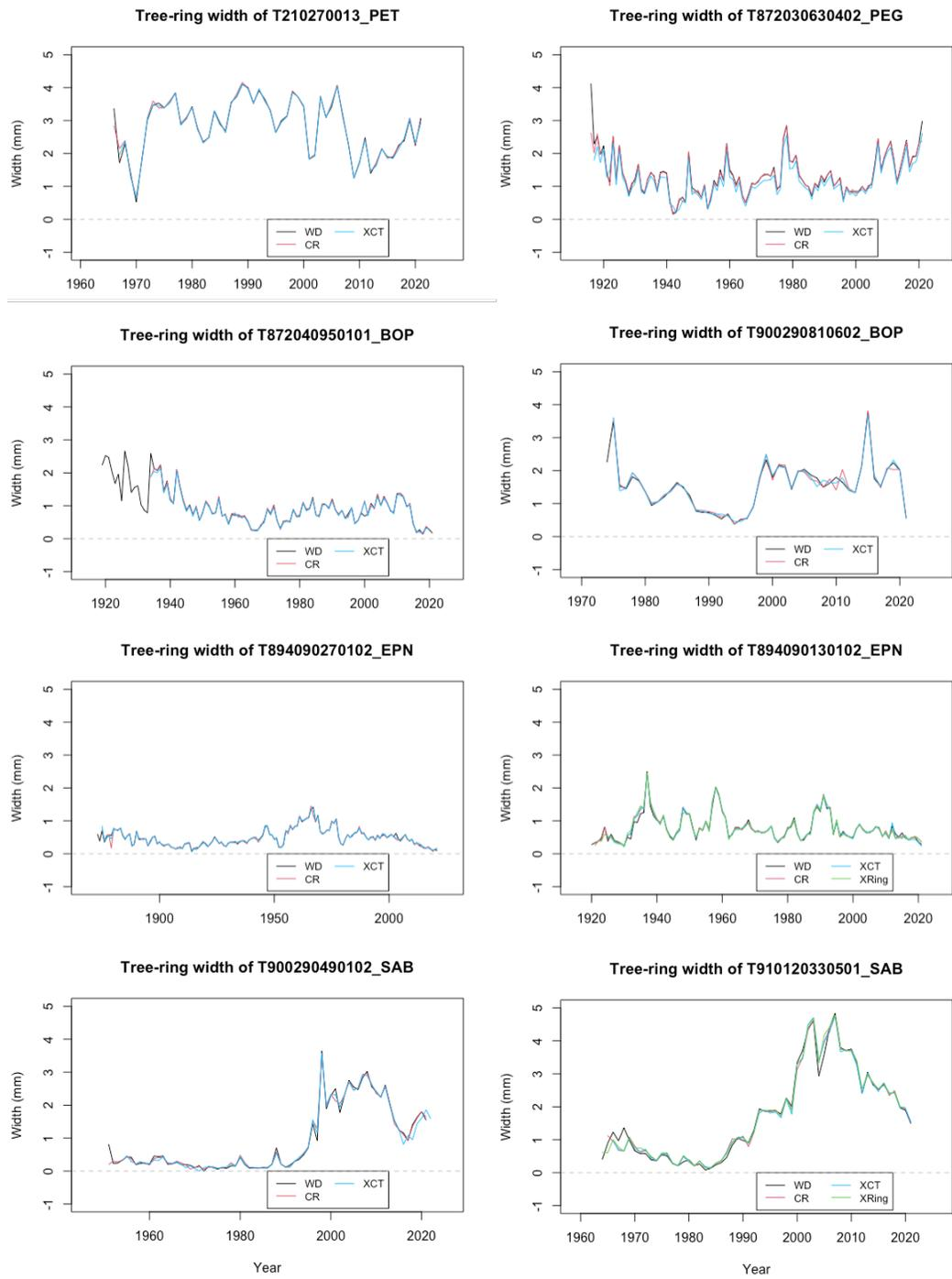
**Figure 6.** Comparison of ring-width measurements of eight selected samples. WD: WinDendro; CR: CooRecorder; XCT: DHXCT; XRing: XRing R package. Note: measurements of DHXCT are generally shorter than those of WD because of the potential “curved ring” issue discussed above.
