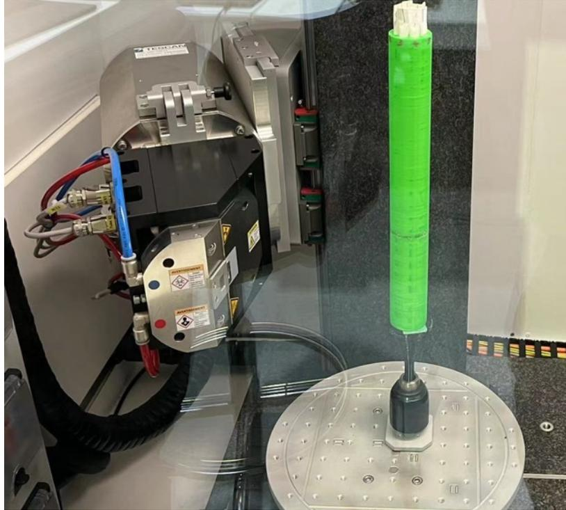
**Figure 2.** Sample holder on the rotating plate. Samples are filled in the green sample holder.
