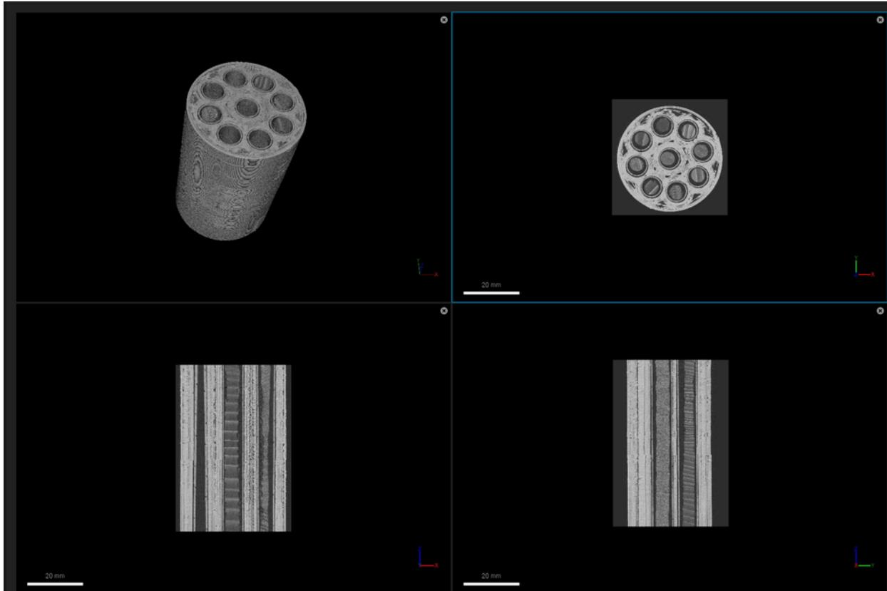
**Figure 3.** An example of one reconstructed 3D image. Wood cores filled in the sample holder can be easily seen.
