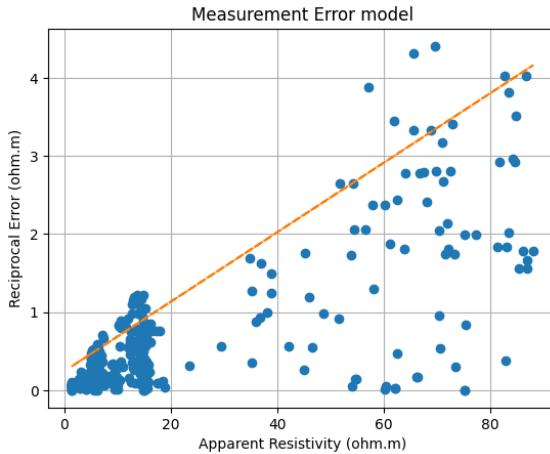
**Figure 2.7 :** The apparent resistivity is plotted versus reciprocal error values to make a linear error model. The linear model is utilized to predict measurement error for each quadrupole.
