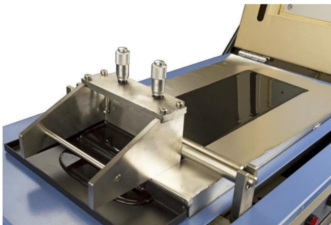
Figure 2.13. The coating process of the ink by the coating machine using Al foil as the current collector.
