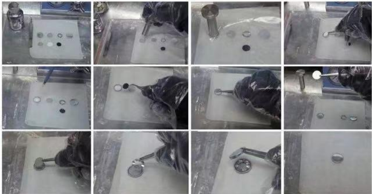
Figure 2.15 The assembling process of Li-ion battery based on a CR2032-type coin cell in an argon-filled glove box.
