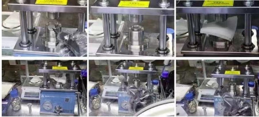
Figure 2.16. The finally sealing process of the Li-ion battery is based on a CR2032-type coin cell in an argon-filled glove box.
