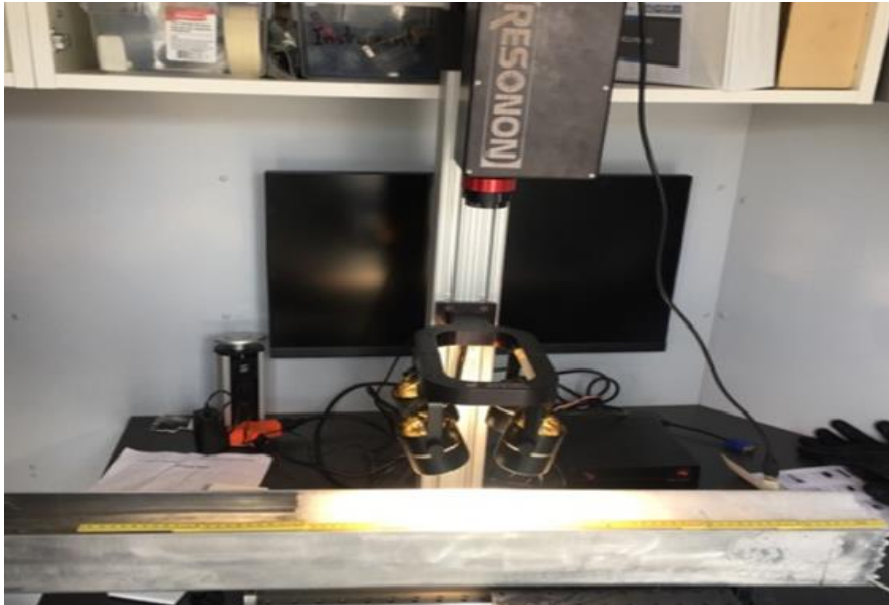
Figure 1-6 : Hyperspectral acquisition of the snow samples vertical profile.
