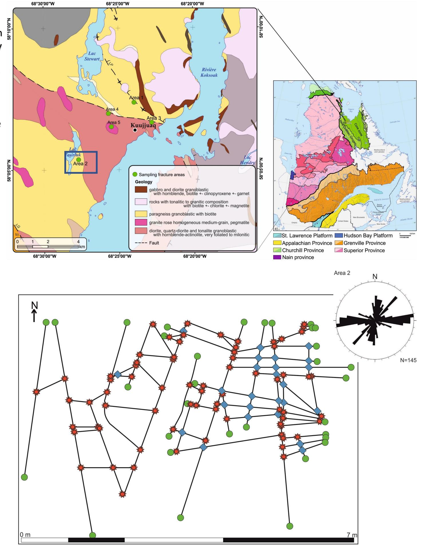
This method enables to qualitatively and quantitatively characterize the fractures and the network properties by recording the different groups of fracture terminations and analyze the data by simple relationships and ternary diagrams.
