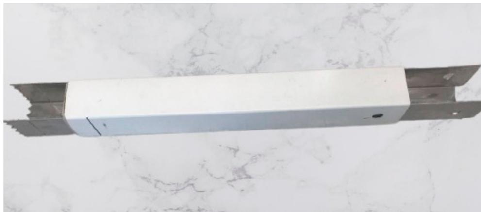
Figure 2. Snow core sampler.
