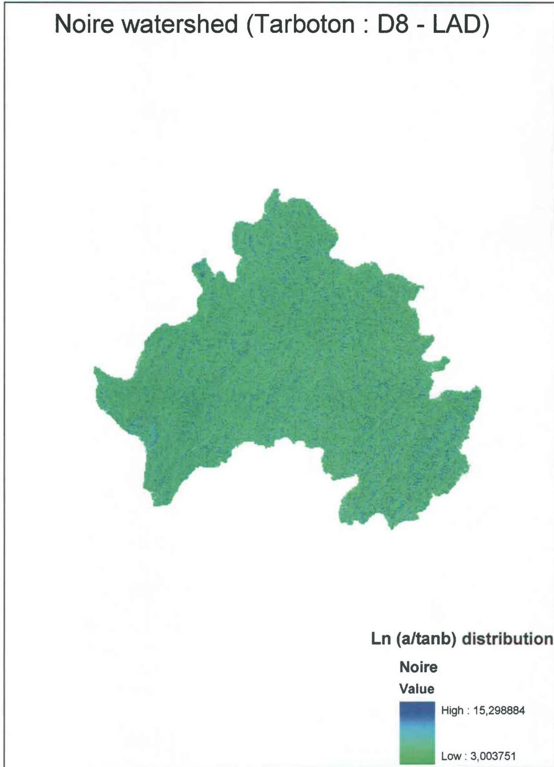
**Figure A.62** : *TI* results for the Noire river watershed using the D8-LAD algorithm (TauDEM)
