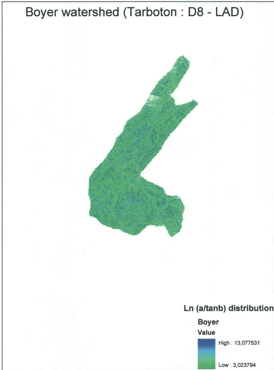
**Figure A.54** : *TI* results for the Boyer river watershed using the D8-LAD algorithm (TauDEM)
