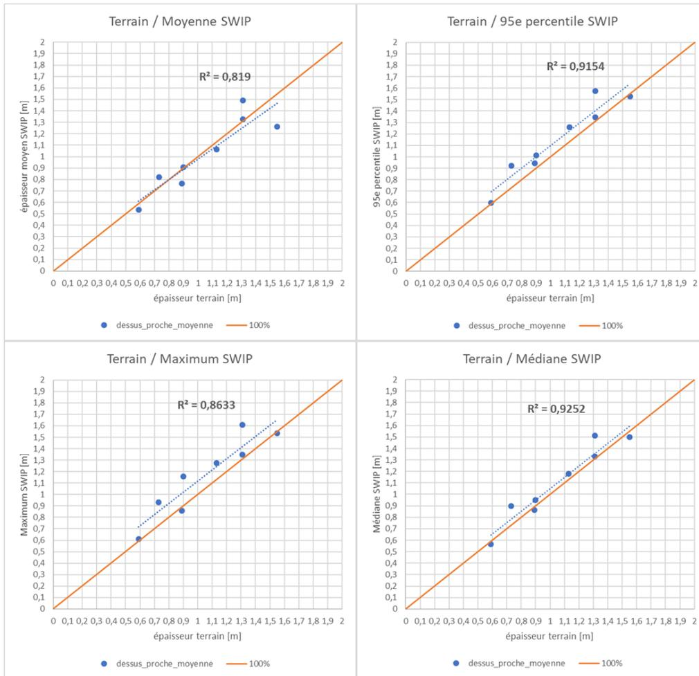
Figure 11: A plot of field measurements with SWIP estimations over 2015-2019 for different filters. Values on the X-Axis are field measurements of ice thicknesses, which depending on the campaign, could have been taken over the instrument, near the instrument or from an average of the area.
