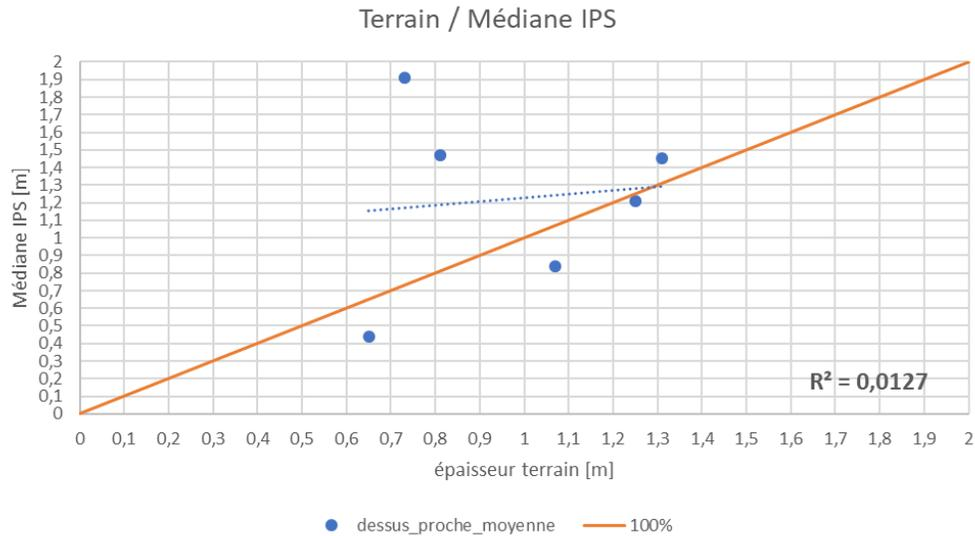
Figure 15: A plot of ice thickness field measurements with IPS estimations over 2016-2019 with the median filter.
