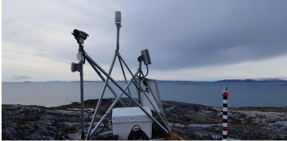
**Figure 25: Camera system with weather station at Niaqurnaᑦ near Kangiqsujuaq**
