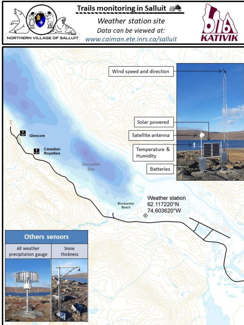
**Figure 26 : Components of the main weather station in Deception Bay**
