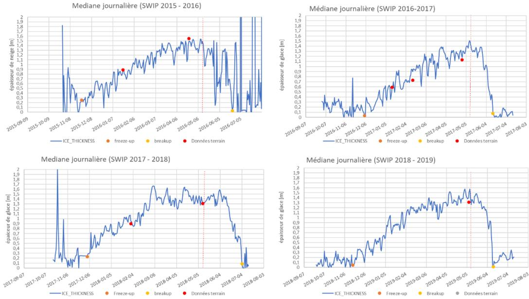
Figure 12: Ice thickness time series (SWIP) for 2015-2019 using the daily median filter
