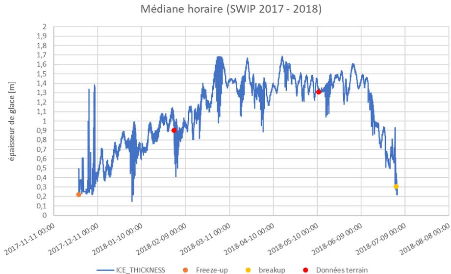
Figure 13: Ice thickness time series (SWIP) for 2017-2018 using the hourly median filter
