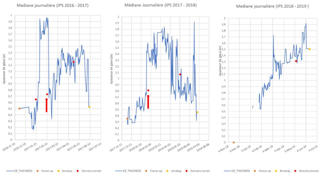
Figure 16: Ice thickness time series (IPS) for 2016-2019 using the daily median filter
