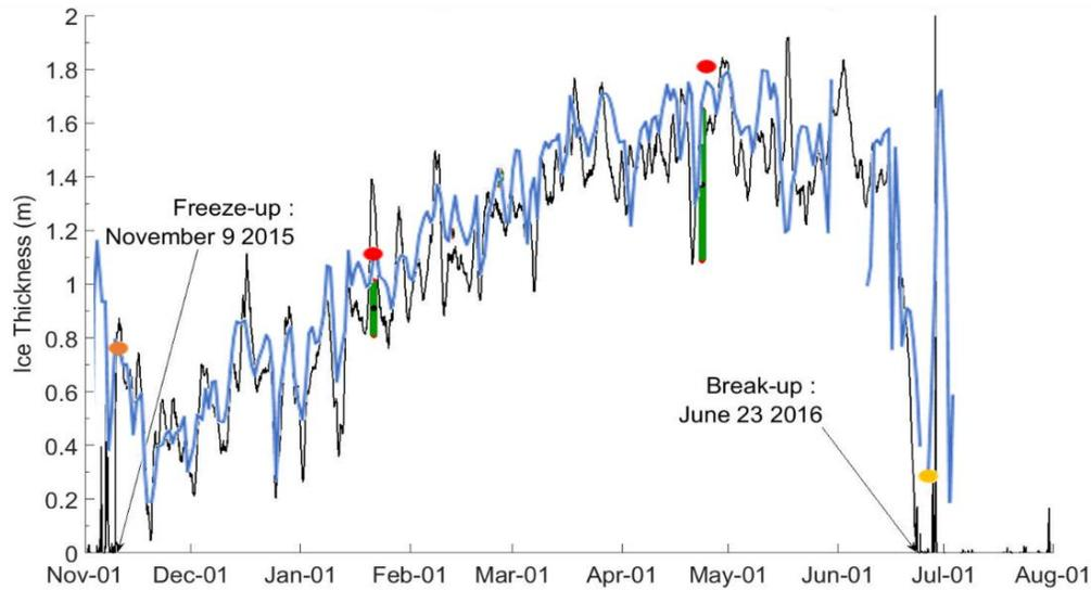
Figure 14: Comparing ice thickness time series (SWIP) for 2015-2016 from complex processing (black line) and simplified processing with daily median filter (blue line)
