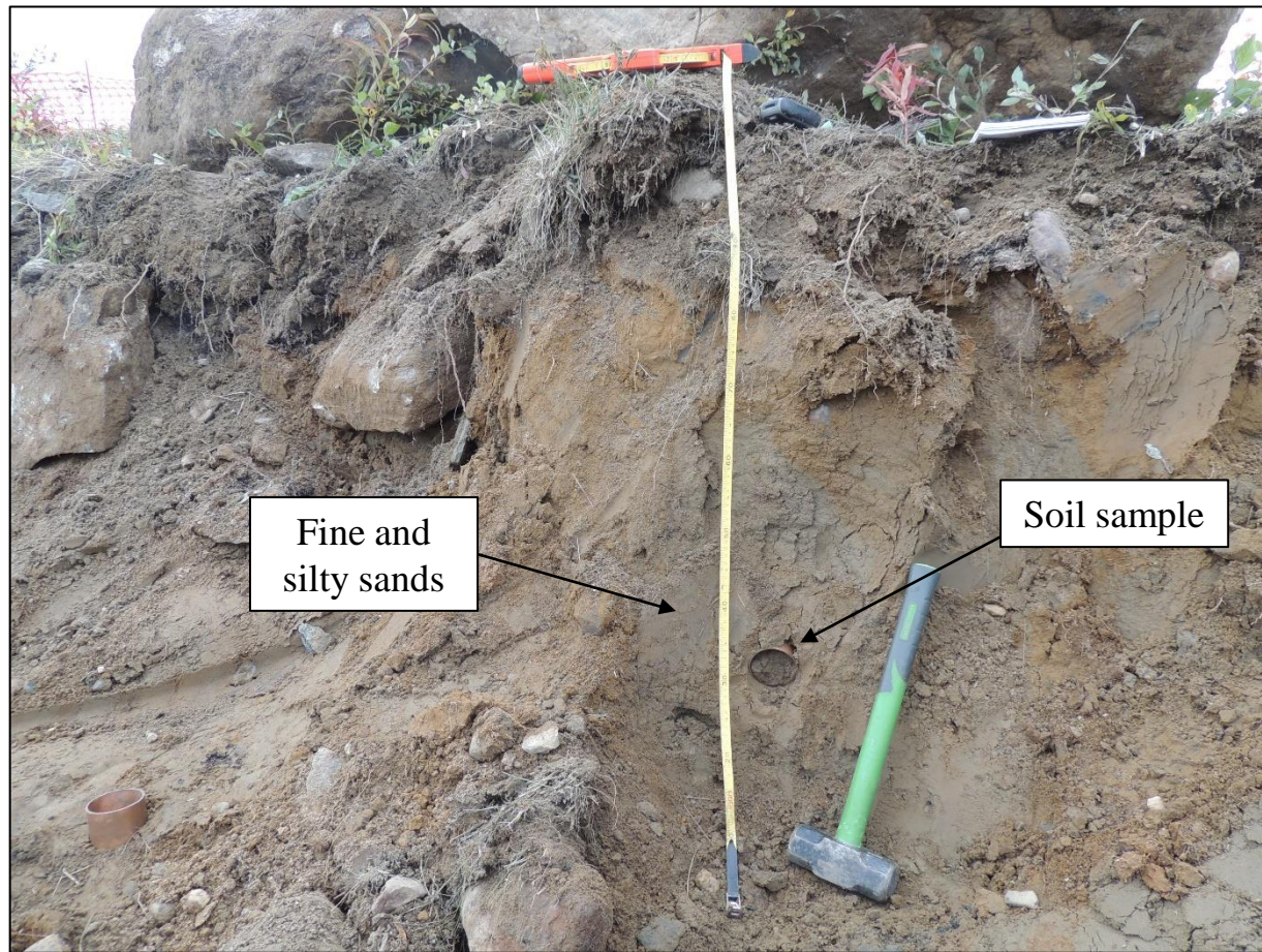
Figure 22 – Geological observation n. 10 with samples of fine sands collected for laboratory analysis of thermal properties .
