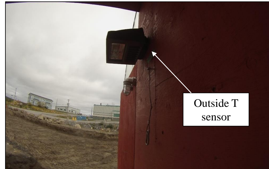
Figure 31 – Inside and outside air temperature monitoring
