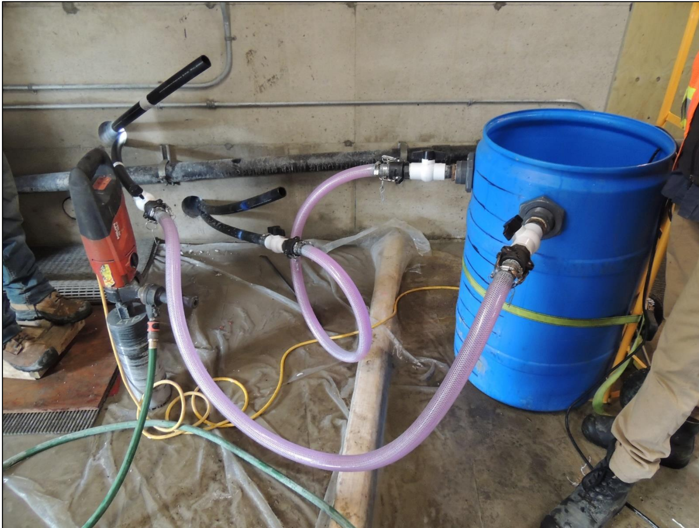
Figure 13 – The mixture of water and antifreeze is injected in one of the 8 loops (left). Technical details of the propylene glycol (right).
