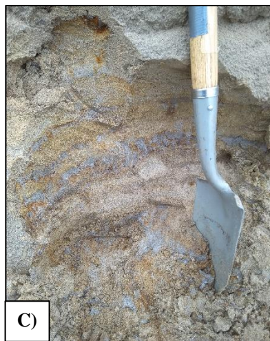
Figure 11 – Sampling of rock formations (A) and unconsolidated sediments (B, sandy delta deposits; C, loamy-sandy marine deposits). D) Analysis of thermal conductivity and volumetric heat capacity of unconsolidated sediments with the needle probe KD2 Pro.
