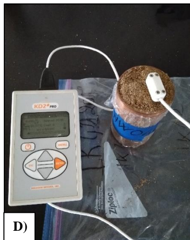
Figure 11 – Sampling of rock formations (A) and unconsolidated sediments (B, sandy delta deposits; C, loamy-sandy marine deposits). D) Analysis of thermal conductivity and volumetric heat capacity of unconsolidated sediments with the needle probe KD2 Pro.
