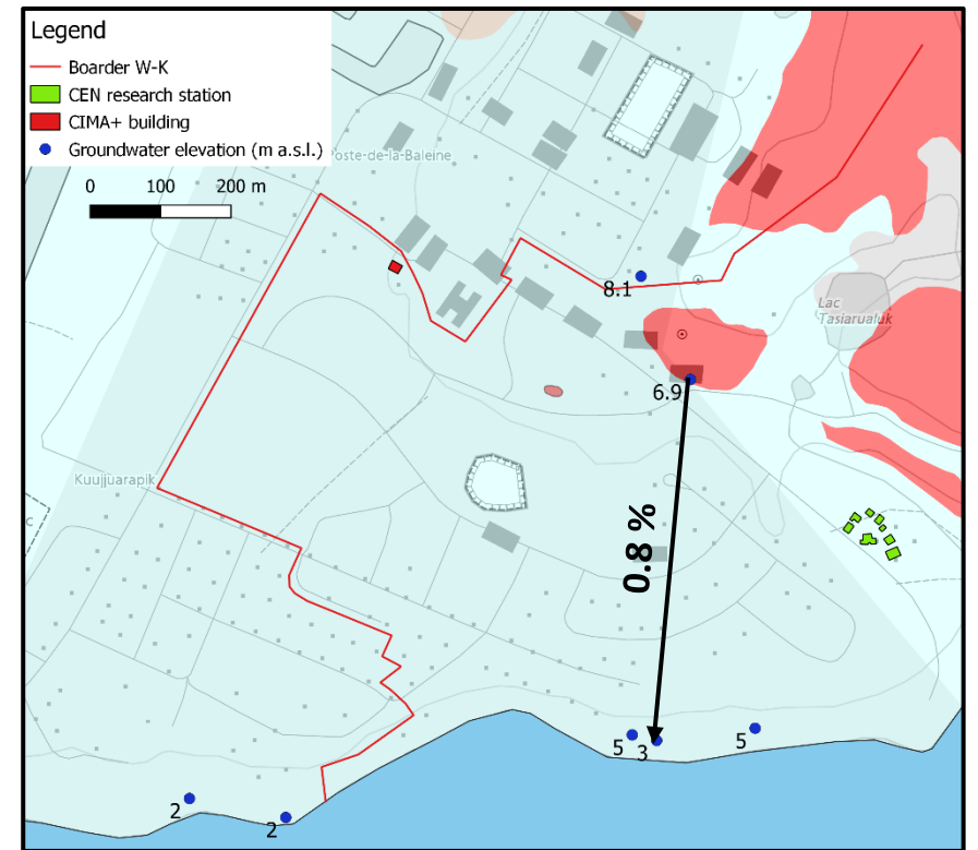
Figure 20 – Location of the available groundwater elevation data and indication of the maximum hydraulic gradient expected at the site (Scale 1:6000).
