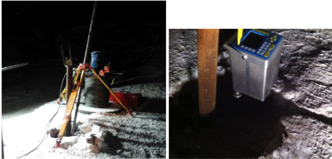
FIGURE 3.9 : Gravilog probe and the surface CG-5 gravimeter taking readings at the surface of the borehole
